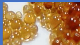
Extract organics from Ion Exchange Resin (UPW 80°C, 7 days)
