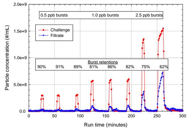
**Ultrafiltration/Microfiltration particle retention:** An example of the retention of 12nm particles by the series combination of a UF module followed by an MF cartridge with a constant challenge concentration is shown in Figure 7. The retention of the UF module was initially about 99% and decreased to less than 97% by the end of the test. Overall retention by the combination of UF and MF remained above 99% throughout the test.
