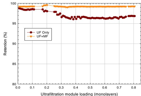
Two additional tests were performed with a combination of UF and MF and constant challenge concentration. Overall, 2 UF cartridges and 3 MF cartridges were used in these evaluations. Table 3 summarizes the retention efficiencies measured at the point in the tests when the UF loading was 0.5 monolayers. UF retention varied from 96.5% to 99.3% while the overall retention efficiency downstream of the MF was >99% in all cases.
